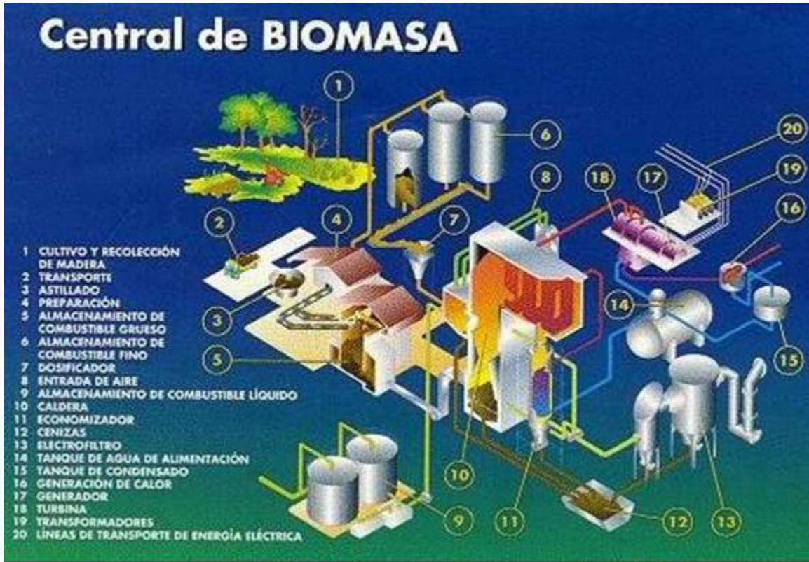
Fig.1.23 Central de Biomasa
